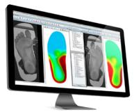
3. AUTOMATIC GENERATION OF MATCHING 3D BOTTOM PROFILES FROM THE MODELLED SURFACE All foot shapes can be milled on both sides regardless of shape
